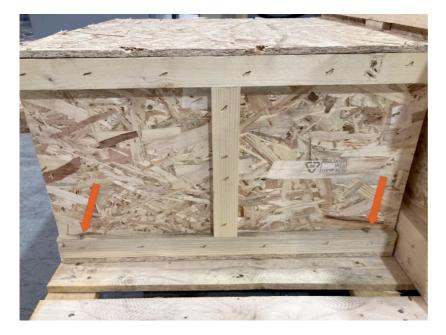
The packaging is fixed to the pallet with fixing stops. Remove them before attempting to move it.
