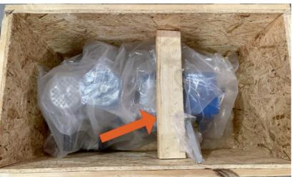
To unpack the deburring machine, first remove the wooden blocking pieces.
