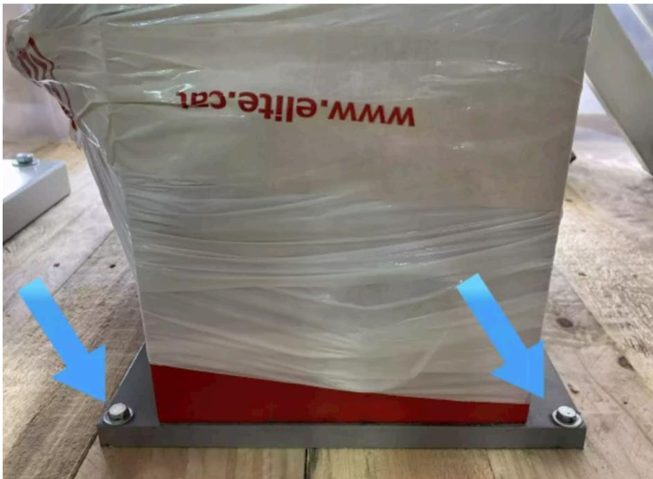
**Once the machine has been moved to its final work destination, you must secure the machine to the ground using the 4 screws placed on the base support of the machine.**
