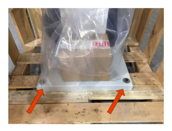
Once the machine has been transferred to its final work destination, you must fix the machine to the ground using the 4 screws placed on the base support of the machine. If this is not done, there is a high risk of the machine tipping over and causing serious injury to personnel and the machine itself.
