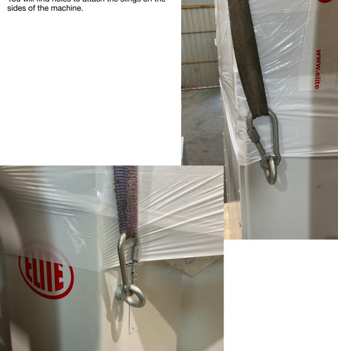
Before connecting the machine, remove any protection that the machine may have to protect the components during transport.
